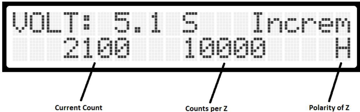
The polarity of Z show the first change in state for the Z signal. If the Z is normally low, it will pulse high and show an “H” there.
