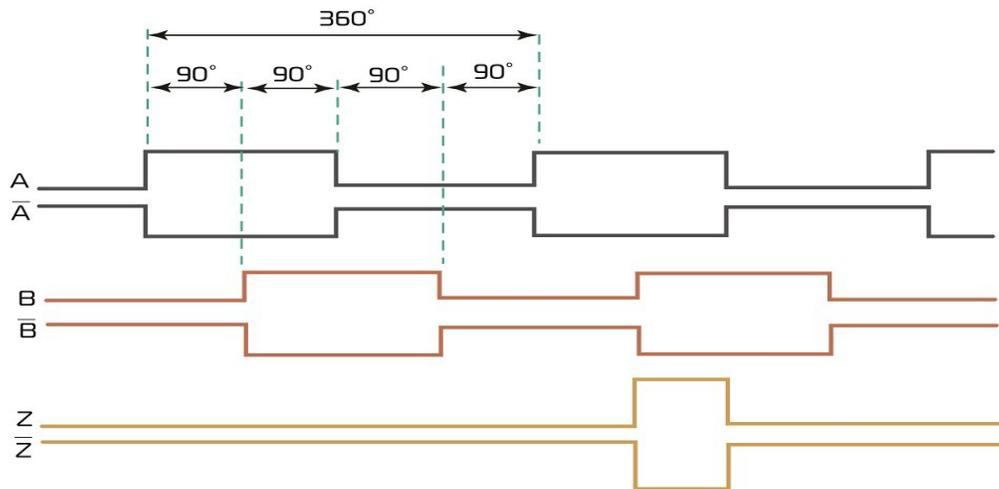
To test this type of encoder, connect the power, ground, A, B, Z (if used) and (if present) the complements A-, B-, Z-. The types of test are:
